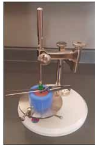
Figure (1): Mono-implant embedded in acrylic resin blocks with the aid of a dental surveyor.
