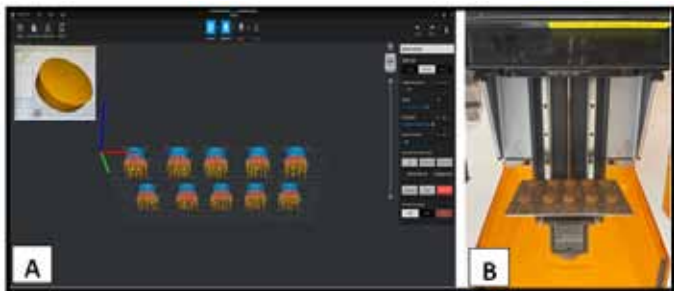
Figure(1): Ten identical specimen configurations A, designed using CAD, and B, printed in the DLP printer's build platform
