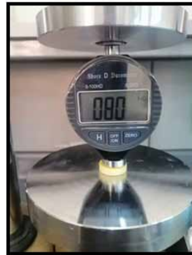
Figure (4): Specimen under surface hardness (Shore D) tester unit
