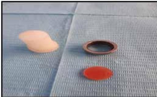
**Figure (1): Metal mold for wax disc specimen fabrication.**
