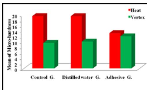
**Figure (3): Mean value of micro-hardness for heat and vertex denture base material.**
