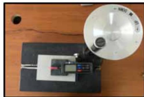
**Figure (3): Profilometer device.**
