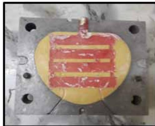
**Figure (2): The flask after injection.**
