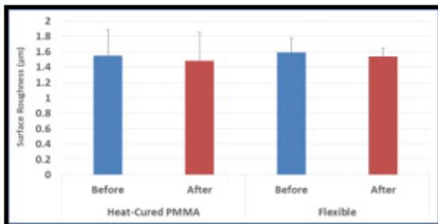
**Figure (5): Bar-chart for the surface roughness of heat-cured acrylic and flexible resin before and after disinfection.**
