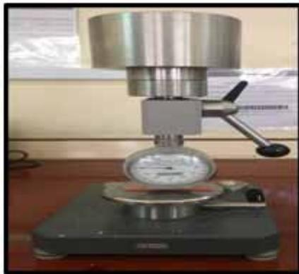
**Figure (4): Shore D hardness tester.**
