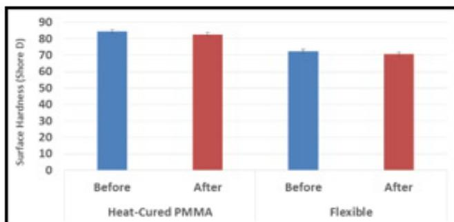
**Figure (6): Bar-chart for the surface hardness of heat-cured acrylic and flexible resin before and after disinfection.**
