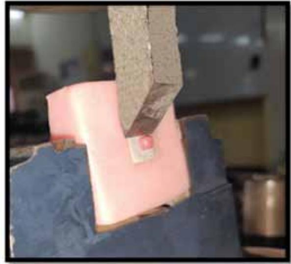
**Figure (4): Specimen under SBS test.**
