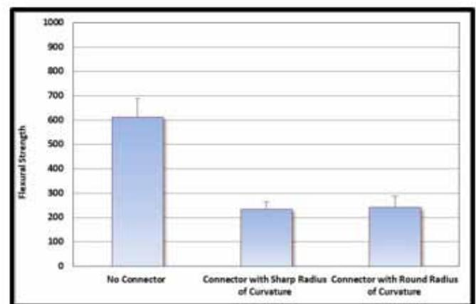
**Figure (3): Bar-Chart showing the mean value of the 3 points flexural strength according to connector's radius of curvature (design).**
