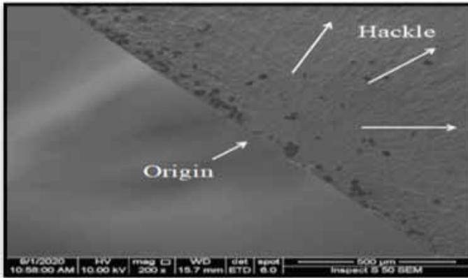
**Figure (4): SEM demonstrating the stress origin and hackle radiations in the fracture surface of zirconia specimen (magnification, ×200).**
