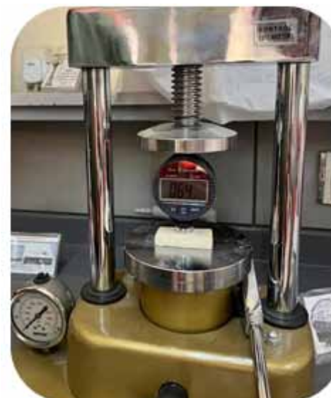
Figure (4): The specimen under surface hardness (shore D) testing unit.
