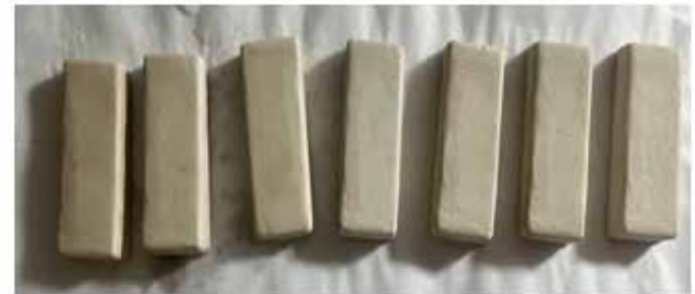
Figure (3): Specimens after dipping in Besswax.
