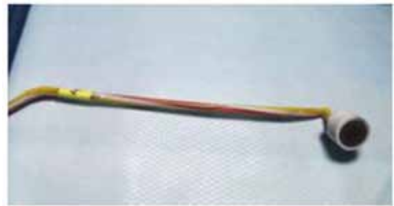
Figure (5): A cylindrical sample mounted by epoxy resin and connected with copper wire.
